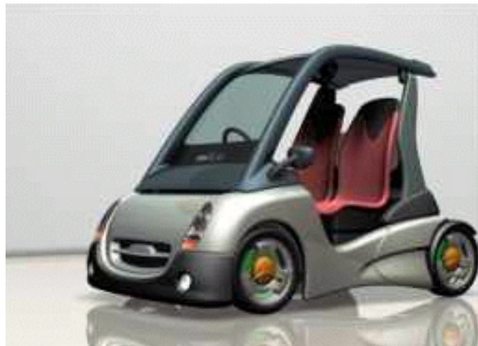
Design Interface (Kowloon, Hong Kong) uses Unigraphics from concept design to final production. Representing a neighborhood electric vehicle designed to ease traffic congestion and pollution, this "mico" concept car was modeled in Unigraphics.
