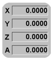
The **POSITION DISPLAY** reflects the present location of each axis in relation to the existing software home, either while jogging or during a program run. The position number tells you how many units away from the software home (in either direction) the axes are.
