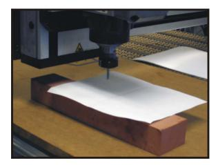
C. Using the Z Jog Buttons to jog the Z-axis down about 1/4 to 1/2-inch above the paper.
