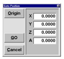
The **GOTO** button window allows you to move any axis to a specified location or move all of them to the machine Origin by pressing Origin.
