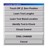
In Step 5-C the Z-axis will start to descend. Normally, you would wait until the Z-axis brings the tool bit to the touchpad and then, if working properly, the Z-axis would retract. For our test, however, we want you to pick up the touchpad and bring it to the tool holder right after the Z-axis begins its descent (see picture below). If the touchpad is working properly, the Z-axis will retract as soon as it makes contact with the tool.
