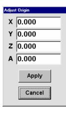
A shortcut window to manipulate the axes position will pop up when you double-click in the Position Display area. The purpose of this window (shown at left) is to be able to tweak the position counters while the program is in Pausemode. After you make the changes you want, click the Apply button and the changes will be made when after the window closes.
