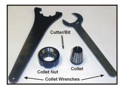
Warning: Turn OFF power to the spindle before removing or replacing the collet!
