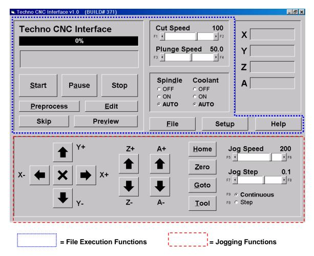
The Techno CNC Interface Main Menu is extremely user-friendly. It is the menu you will see and use the most. The Main Menu allows you to Select, Start and Pause a file; Home and Zero the machine; adjust Speeds and Spindle controls and much-much more.
