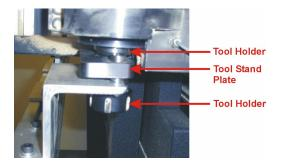
Warning: DO NOT go more than 3 clicks down on the Tool stand Plate (using a 0.01 Jog Step).
