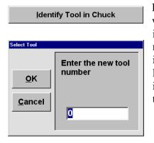
Press **THE IDENTIFY TOOL IN CHUCK** button when you need to identify the tool in the chuck. For instance, if after a software crash, the Interface does not remember what number tool is in the chuck, the interface, however, does remember the tool stand locations. So, if you input the tool number into the input box (shown at right) you will be able to return the tool to the proper tool stand.
