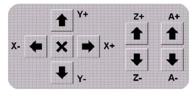
Each axis has specific arrow buttons that will move (or jog) the axis in either a positive or negative direction. The value of the letter (= or -) designates in which direction that arrow will jog the axis. There are three sets of jog buttons: the X/Y-axes buttons, the Z-axis buttons and the A-axis buttons.
