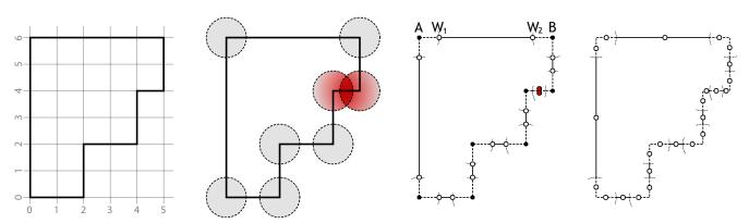
The first image shows our input curve positioned on a unit grid. The shortest segment has a length of 1.0, the longest segment a length of 6.0. If we're going to blend all corners with a radius of 0.75 (the circles in the second image) we can see that one of the edges has a conflict of overlapping blend radii.
