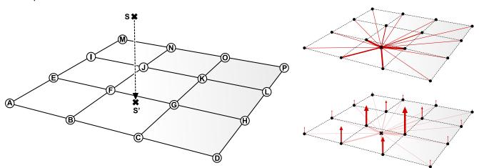
For purposes of clarity I have unfolded a very twisted nurbs patch so that it is reduced to a rectangular grid of control-points. Actually, I'm making this up as I go along, I haven't really unfolded anything but I need you to realize that the diagram you're looking at is drawn in {uvw} space rather than world {xyz} space. The actual surface might be contorted in any number of ways, but we're only interested in the simplified {uvw} space.
