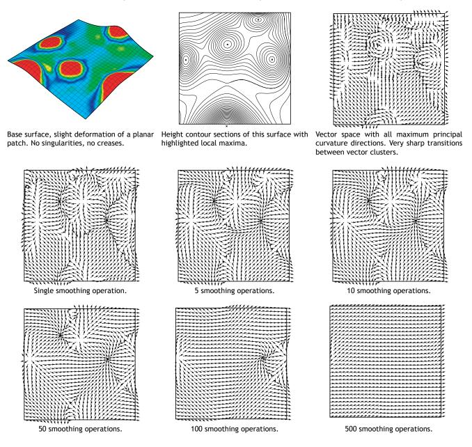
This progression of smoothing iterations clearly demonstrates the usefulness of a tensor-smoothing algorithm; it helps you to get rid of singularities and creases in any continuous tensor space.
