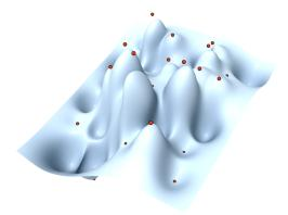
The first iteration started with a flat surface, with all the normals pointing directly upwards. However, after the control-points were adjusted, the surface is far from planar. Since we restrict Control Point motion along the normal of the Greville Point, the surface now starts to bulge horizontally as well. Deviation reduced to 34mm.
