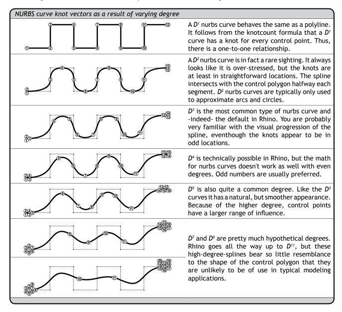
A clamped curve always has a bunch of knots at the beginning and end (periodic curves do not, but we'll get to that later). If a curve has knot clusters on the interior as well, then it will touch one of the interior control points and we have a kinked curve. There is a lot more to know about knots, but we're already dangerously close to permanent brain injury so I suggest we continue with some simple nurbs curves and let Rhino worry about the knot vector for the time being.
