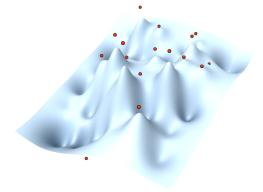
This image is recognizable as a 3D version of the diagrams you've seen before. Every point has a small summit pointing towards it. This is the result of the first iteration of our algorithm. Total deviation is still 63mm (measured as total distance between all red points and their projection onto the surface).
