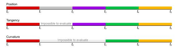
When using curve properties such as tangents, curvature or perp-frames, we must always be careful to not blindly march on without checking for property discontinuities. An example of an algorithm that has to deal with this would be the *\_CurvatureGraph* in Rhino. It works on all curve types, which means it must be able to detect and ignore linear and zero-length segments that lack curvature.
