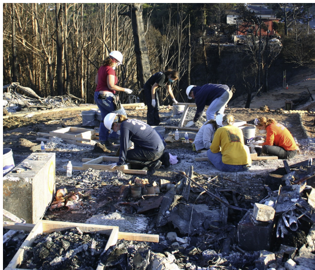
FIGURE 6.23 Screening debris from fire scene
