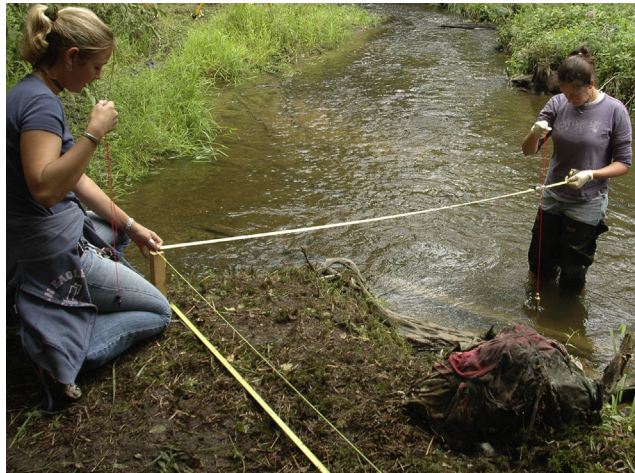
FIGURE 6.10 Plumb-bob used to take a vertical measurement
