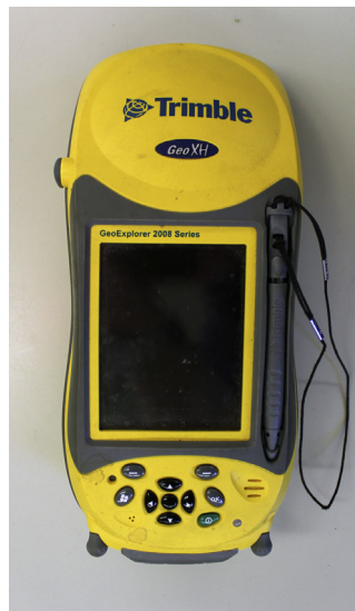
FIGURE 6.18 Global positioning system (GPS) device
