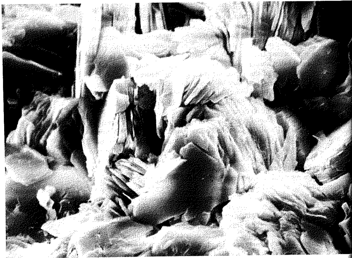
Figure 2.6 Platelets of kaolin clay, as seen in a scanning electron microscope under 3,700x magnification. Although individual particles may be less than half a micron thick, they frequently occur as stacks of platelets that require
