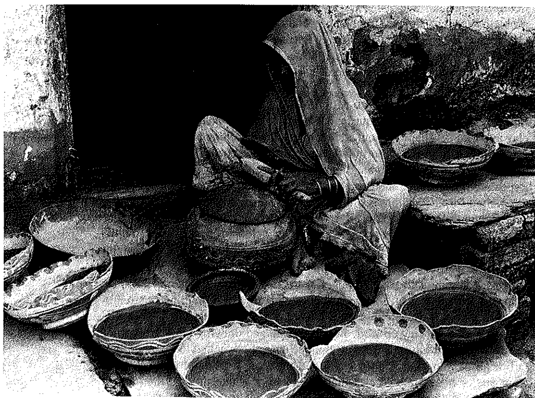
Figure 5.3 A woman belonging to a potter caste in Udaipur, Rajasthan, India, making griddles by paddling clay over the base of a water storage jar. The griddles are then dried
