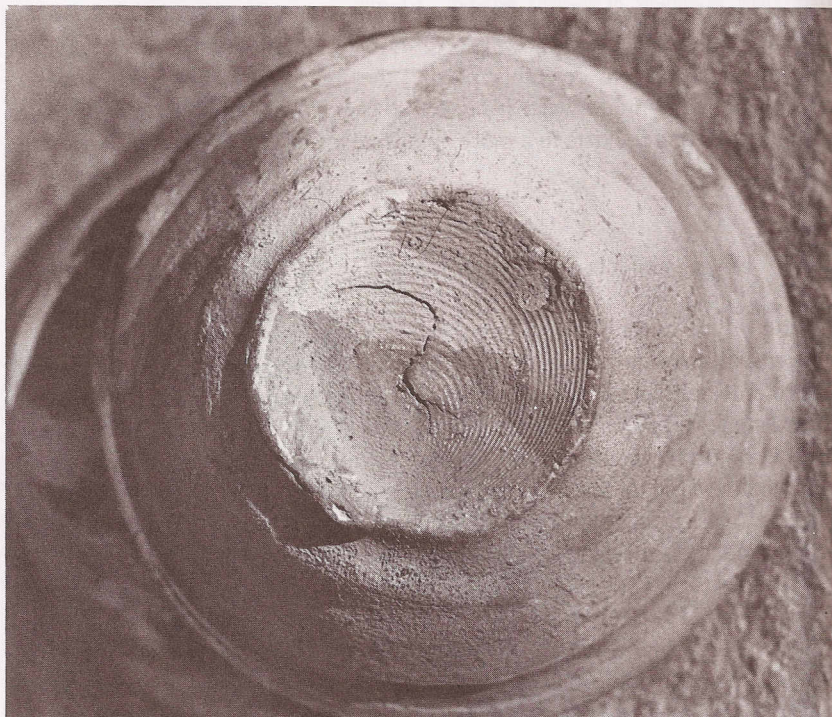
Figure 3.6 An S-shaped crack on the base of a small wheel-thrown ashtray, a typical drying defect (exaggerated in firing) caused by differential water and resultant uneven shrinkage.
