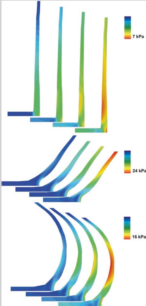
**Fig. 2.34** Repartition of the mechanical stresses inside the walls of the cylinder, bowl, and sphere, for the 2.25 kg pots. From left to right, the rotation speed is 0, 120, 160, and 200 rotations/min. The change in stresses distribution observed here (on the 2.25 kg pots) is qualitatively similar to that of the 0.75 kg pots. The geometry of the vase being very close to that of the sphere, we have not presented it here
