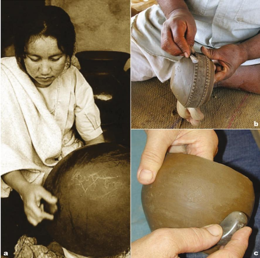
**Fig. 2.46** Examples of surface treatments: (a) and (c) burnishing with a pebble (Manipur, India; Experimental Center of Lejre, Denmark); (b) softening with a piece of wood (Udaipur, Gujarat, India)
