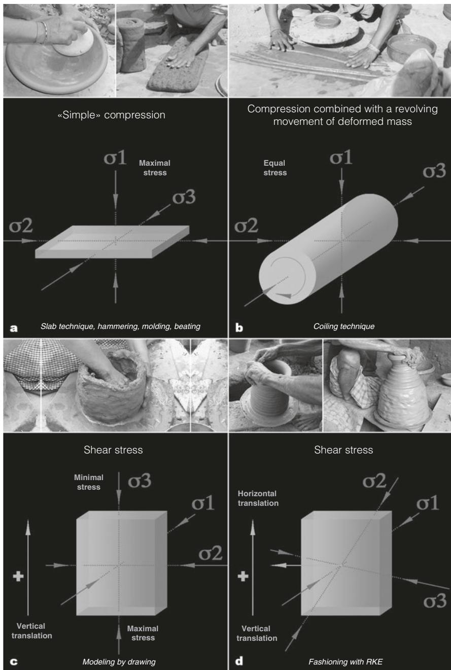
**Fig. 3.20** Theoretical classification of the mechanical stresses associated with the different fashioning techniques (after Pierret 2001): (a) planar anisotropy (flattening along the plane perpendicular to the axis of maximal stress); (b) linear anisotropy (drawing along the axis of minimal stress); (c, d) plano-linear anisotropy (drawing along the axis of minimal stress and flattening along the plane perpendicular to the axis of maximal stress)
