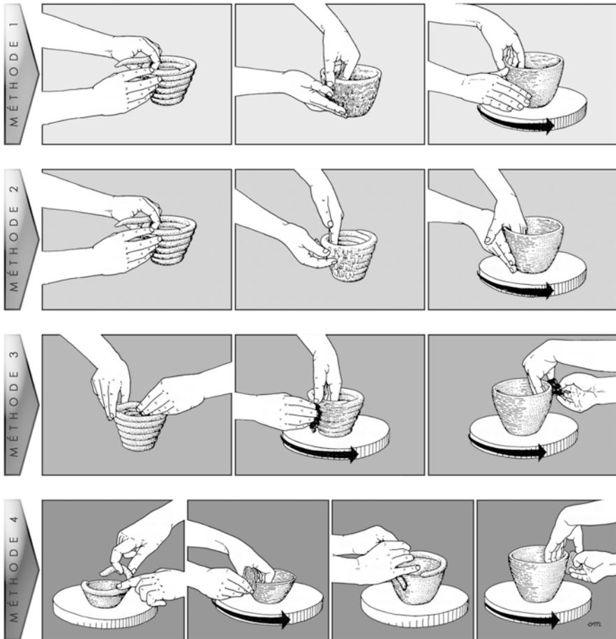
Fig. 2.37 Illustration of the four wheel coiling methods. (After Roux and Courty 1998)
