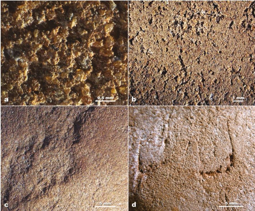
**Fig. 3.39** Diagnostic features of beating: (a) micro-pull-outs; (b) surface with inserted grains, compact microtopography, and micro-pull-outs; (c) percussion cupule traces with irregular contours; (d) fissure due to vertical external percussion blows on a heterogeneous base (made from patches of clay) and presence of ash as anti-adhesive
