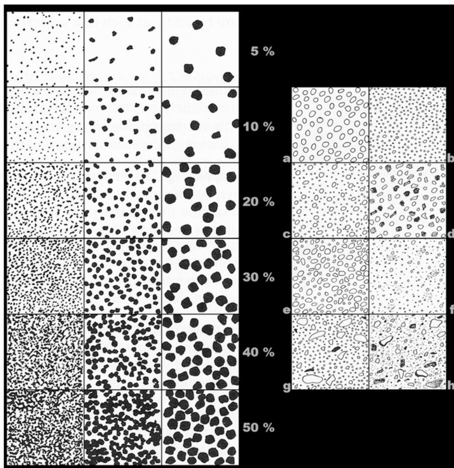
Fig. 3.3 Quantification charts (after Courty et al. 1989): (a) chart used to estimate the abundance of the coarse fraction in the fine mass; (b) chart used to estimate the degree of roundness of the coarse fraction in the fine mass
