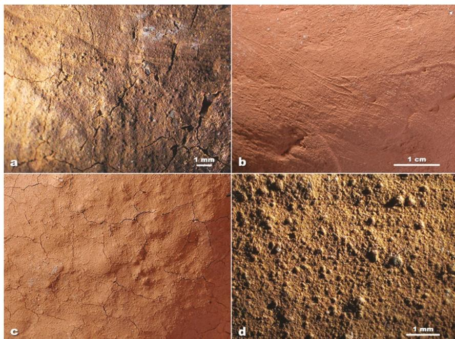
**Fig. 3.58** Examples of clay-coated surfaces: **(a, b)** overthicknesses and floating grains; **(c)** clay coating applied with a wooden tool on wet paste; **(d)** clay coating applied with a piece of leather on leather-hard paste
