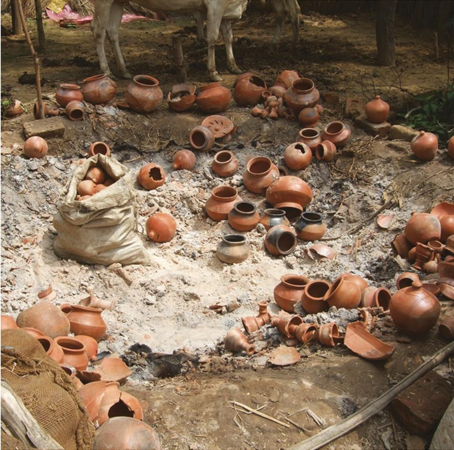
**Fig. 2.57** Open firing in depression and firing accident due to gusts of wind (Dibai, Uttar Pradesh, India)
