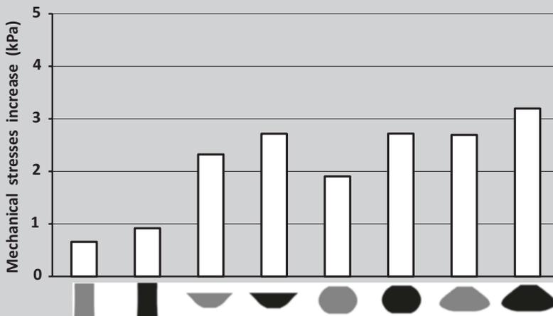
**Fig. 2.35** Increase of the maximum Von Mises values, for the eight reproductions, from the static situation (zero speed) to the situation where the wheel is activated at 152 rotations/min (for the 0.75 kg pots) and 125 rotations/min (for the 2.25 kg pots). The four forms (cylinder, bowl, sphere, and vase) are represented on the *x*-axis; the pots of 0.75 kg are in gray and those of 2.25 kg in black
