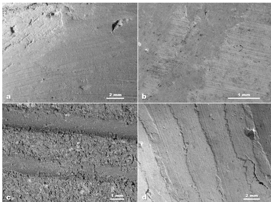
**Fig. 3.55** Examples of surface treatment by friction: **(a)** previously shaved surface softened with a wooden stick loaded with water; **(b)** burnished strips on previously wet smoothed surface; **(c)** burnished strips on leather-hard hammered paste; **(d)** facets with scalloped edges formed during burnishing
