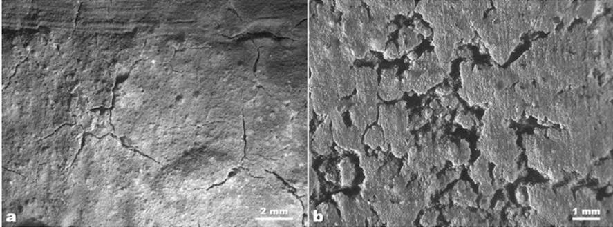
**Fig. 3.10** Examples of cracks and crevices: (a) drying cracks; (b) crevices
