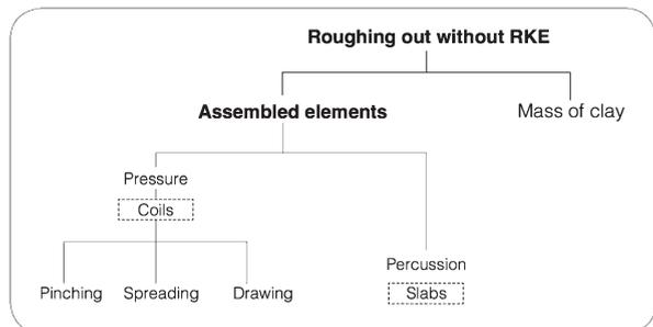
The coiling technique can be used to form the different morphological parts of recipients: the base, body, and neck. The body and the neck are obtained by overlaying the coils on each other in a vertical plane. The base is obtained by adding coils against each other in a horizontal plane.
