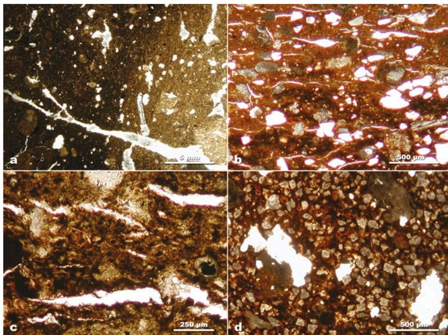
**Fig. 3.21** Illustration of the types of pores often present in ceramic petrofabrics: (a) cracks and cavities; (b) fissures and cavities; (c) cavities and fine fissures; (d) vesicles
