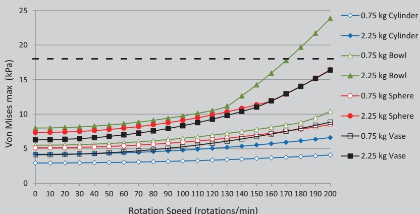
**Fig. 2.33** The Von Mises maximum values for the eight reproductions depending on the rotation speed ranging from 0 to 200 rotations/min. The threshold of collapse ( $18 \pm 2.7$  kPa) is showed by a dotted line
