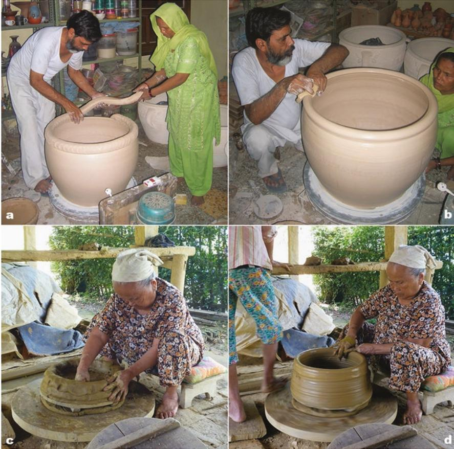
**Fig. 2.36** Examples of wheel coiling: (a) and (b) wheel coiling on electric wheel (New Delhi, India); (c) and (d) wheel coiling on a turntable activated by the helper's foot (Vietnam, ©A. Favereau)
