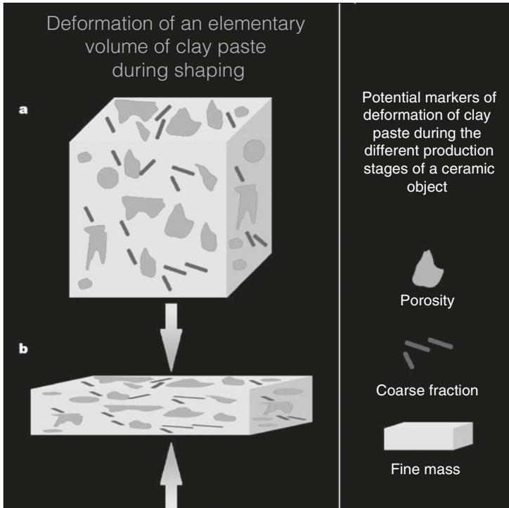
**Fig. 3.19** Simplified view of the deformation of an elementary volume of clay paste (after Pierret 2001). This representation is at a mesoscale and does not take account of the deformations of the clay domains
