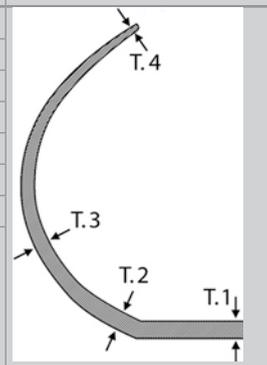
Thickness has been measured at four levels: middle of the base (T.1), bottom of the wall (T.2), middle of the wall (T.3), and top of the wall (T.4)
