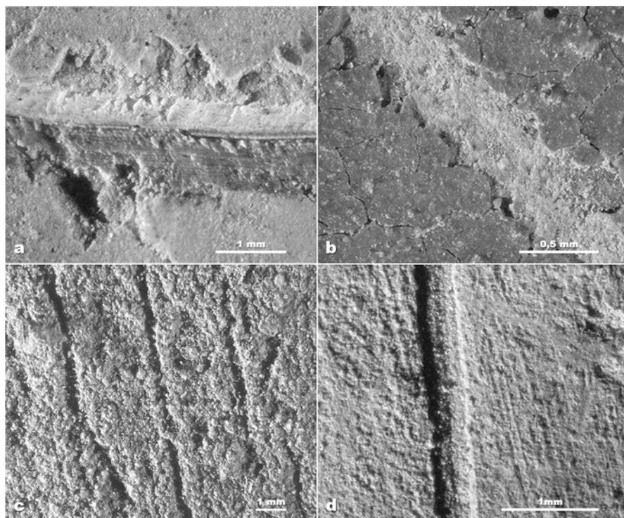
**Fig. 3.18** Edges of striations: (a, b) scaled; (c) irregular; (d) regular
