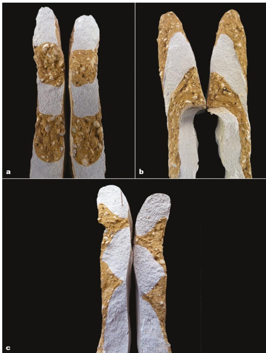
**Fig. 3.26** Examples of joints of coils on experimental material: (a) horizontal and U-shaped joints obtained with coiling by pinching according to non-systematic gestures; (b) beveled joints obtained with coiling by spreading; (c) alternate beveled joints
