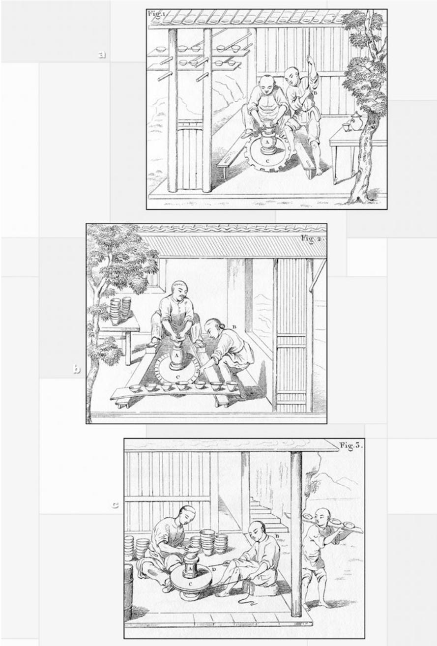
**Fig. 2.14** Different ways to rotate the wheel in China: (a) with assistant's foot; (b) with assistant's hand; (c) with a rope wrapped around the wheel and operated by the assistant in a reciprocating movement (Brongniart 1977 (1877), PL. XLIII)
