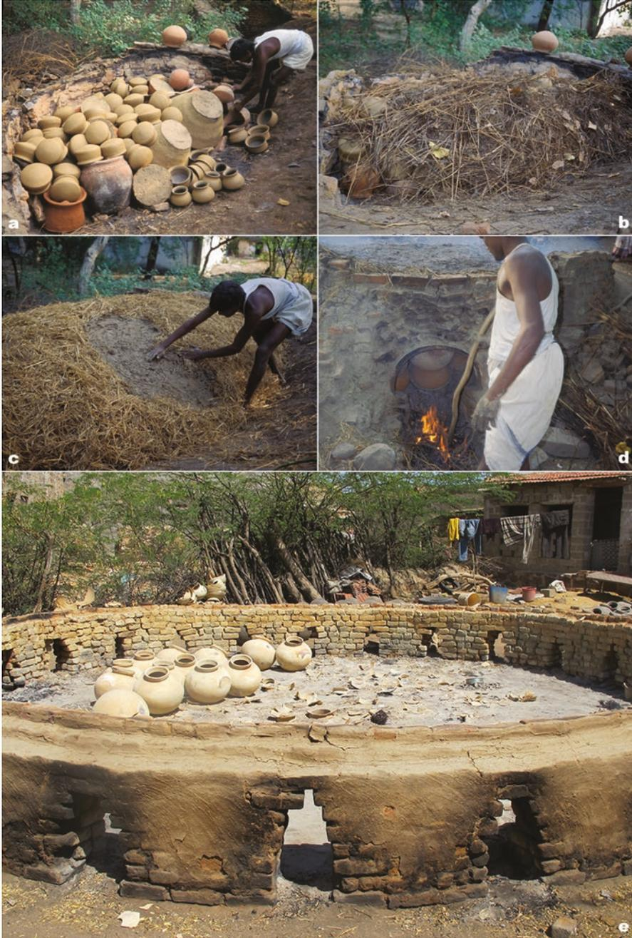
**Fig. 2.55** Enclosed firing: (a) a semicircular wall made of fired bricks block a slope; (b) the recipients are placed on a bed of straw and then covered successively with straw and branches; (c) the structure is coated with wet clay; (d) the firing starts from an opening made in the middle of the semicircular wall and is fueled with branches; it lasts around 5 h and the cooling lasts around 12 h (Andhra Pradesh, India); (e) enclosed firing with multiple openings (Pachpadra, Rajasthan, India)
