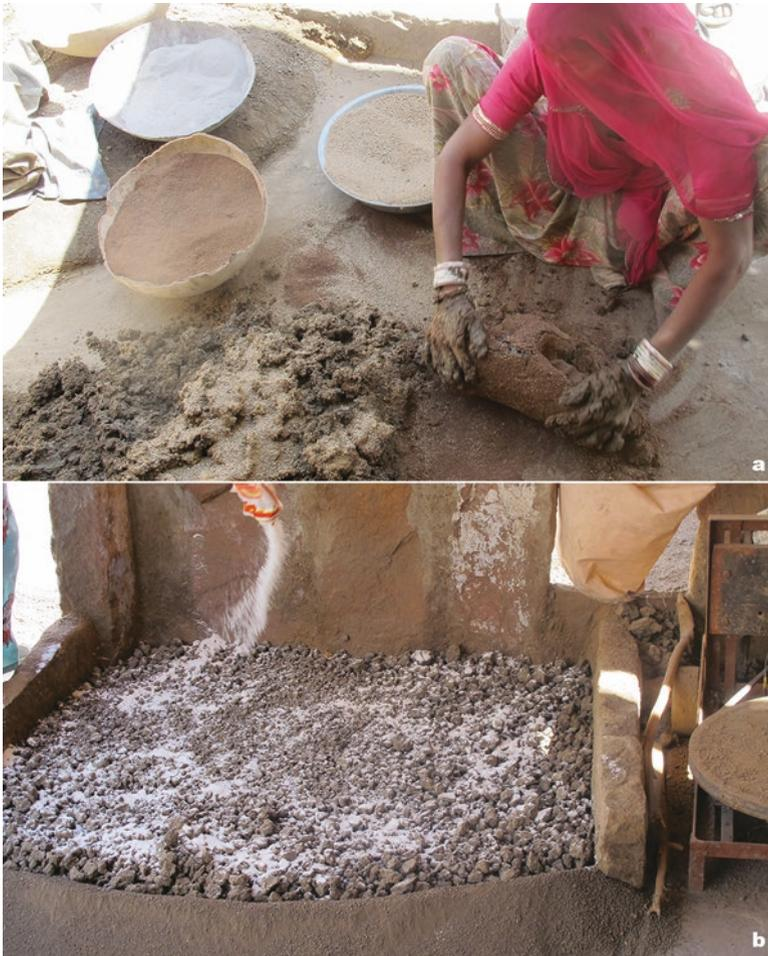
**Fig. 2.8** Adding tempers: (a) adding granite grains and sawdust to hydrated paste during kneading (Salawas, Rajasthan, India); (b) adding salt to the coarse fraction before hydration in order to get “hydroceramic” paste (Salawas, Rajasthan, India)
