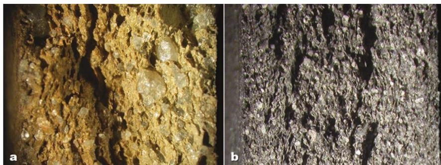
**Fig. 3.31** Diagnostic microstructures of modeling by drawing – networks of elongated fissures and subparallel orientation of the asymmetric coarse fraction: (a) Bantu modeled ceramic; (b) Danish modeled ceramic
