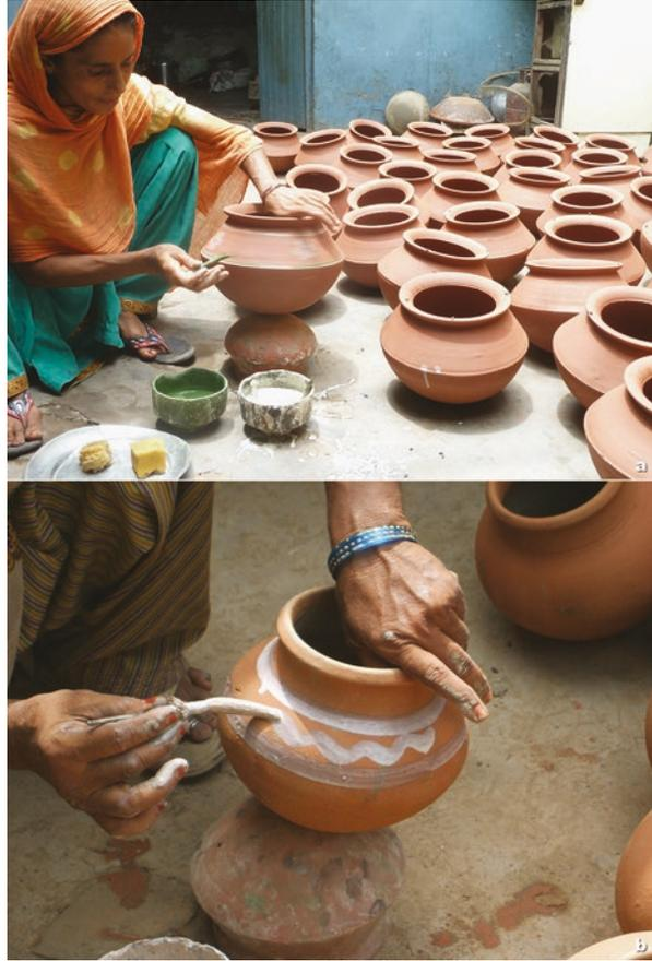
The pigments used in the paints are coloring substances in the form of powder before being mixed with a liquid. They are of mineral or organic origin. Mineral colorings include iron oxides, which produce colors ranging from yellow (greenish to orangey) to different shades of red-brown, manganese oxides for black, metamorphic rocks such as lapis lazuli for blue, or rocks such as kaolinite for white. Organic pigments are extremely diverse and vary depending on the region.
