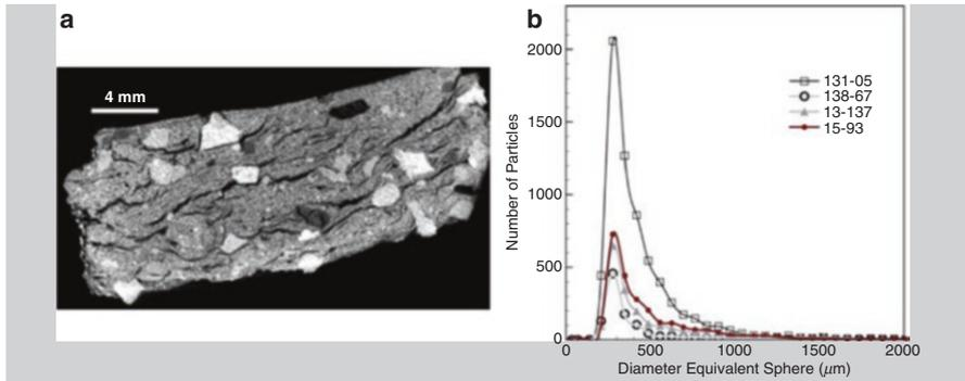
**Fig. 3.51** High-resolution X-ray microtomography ( $\mu$ -CT): (a) reconstructed image of a Neolithic pottery fragment from northern Germany; (b) example of quantitative analysis of four Neolithic shards from northern Germany – abundance of rock fragment temper in different size classes in the Neolithic pottery sherds (after Kahl and Ramming 2012)
