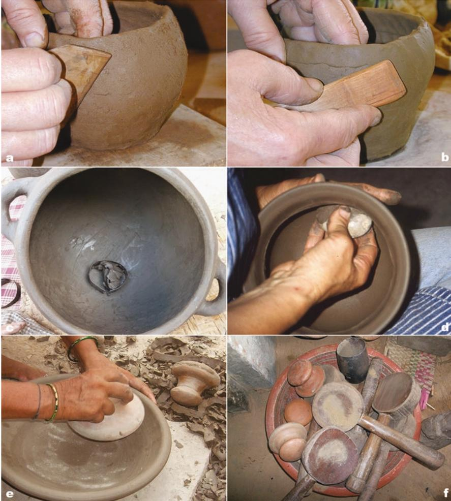
**Fig. 2.10** Examples of active tools: (a) wooden scraper (Experimental Centre of Lejre, Denmark); (b) wooden forming tool (Experimental Center of Lejre); (c) iron shaving tool (Michoacan, Mexico); (d) stone pusher (Experimental Centre of Lejre, Denmark); (e) ceramic tenon hammer (Uttar Pradesh, India); (f) wooden paddles and ceramic tenon anvils (Uttar Pradesh, India)
