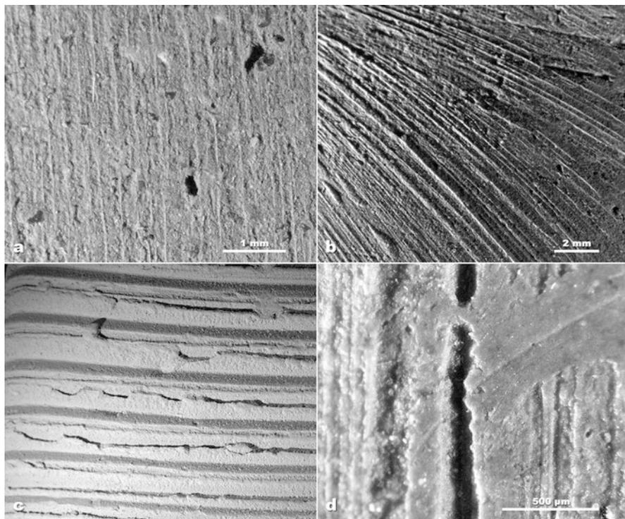
**Fig. 3.17** Edges of striations: (a) threaded; (b) ribbed; (c) thickened; (d) scalloped
