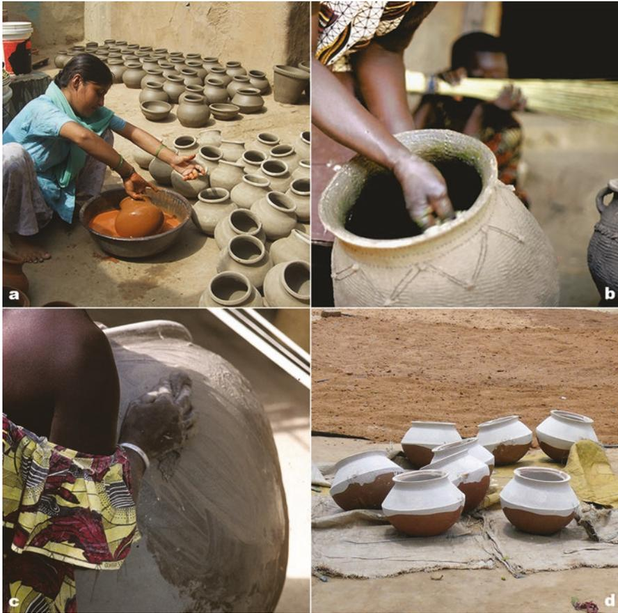
**Fig. 2.47** Example of surface treatments: (a) slipping by soaking (Uttar Pradesh, India); (b) coating with organic material before firing (Senegal, ©A. Gelbert); (c) coating with clay slurry by wiping it on (Mali, ©A. Gallay); (d) coating with glaze on dry slipped and painted cooking pots, before firing (Uttar Pradesh, India)
