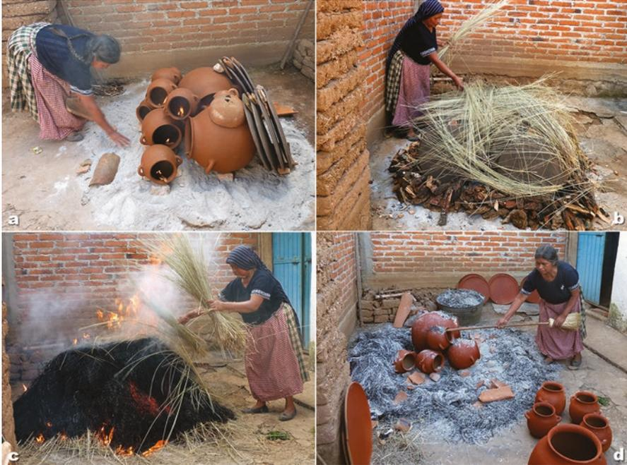
**Fig. 2.54** Pre-heating and open firing: (a) pre-heating recipients placed on a layer of ashes; (b) after the recipients have been covered with cow dung patties, pine bark, and wood, the structure is covered with long dried herbs; (c) the firing is refueled after 7 min; (d) the pots are removed from the firing after 2 h (Michoacán, Mexico)
