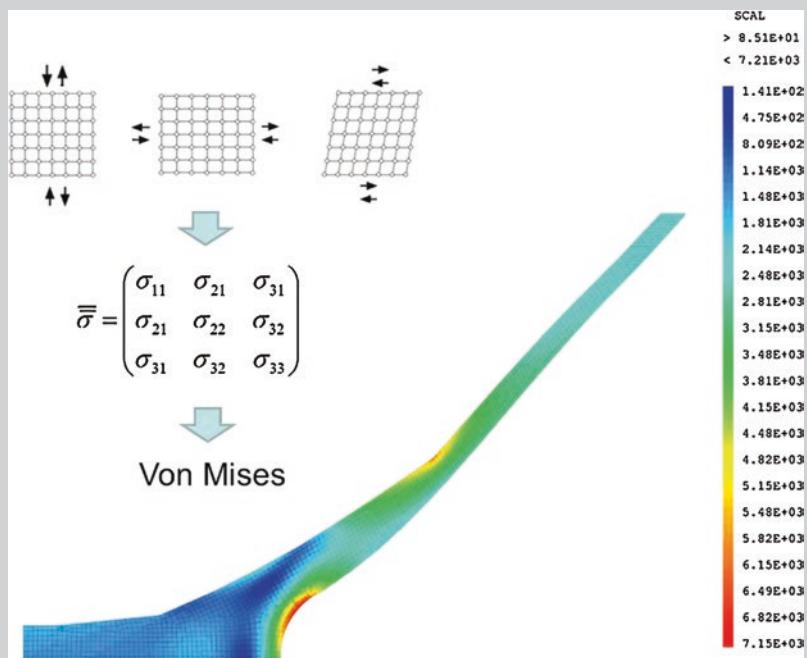
**Fig. 2.32** Cross-sectional 2D profile of a 2.25 kg bowl mechanical modeling. The Von Mises norm synthesizes the matrix of mechanical stresses ( $\bar{\sigma}$ ), and the maximum value of this norm is an overall index of the mechanical state of the pot. This bowl reaches a Von Mises maximum value of 7.13 kPa. The color scale (from dark blue to dark red) represents the increasing values of mechanical stresses. The color mapping shows the distribution of the mechanical stresses inside the walls
