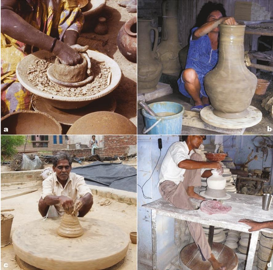
**Fig. 2.12** Examples of rotary instruments: (a) rotary device (Mali, ©A. Gallay); (b) turntable fixed on a wooden plank (Leyte Island, Philippines); (c) simple wheel launched with a stick (Uttar Pradesh, India); (d) double wheel (Uttar Pradesh, India)
