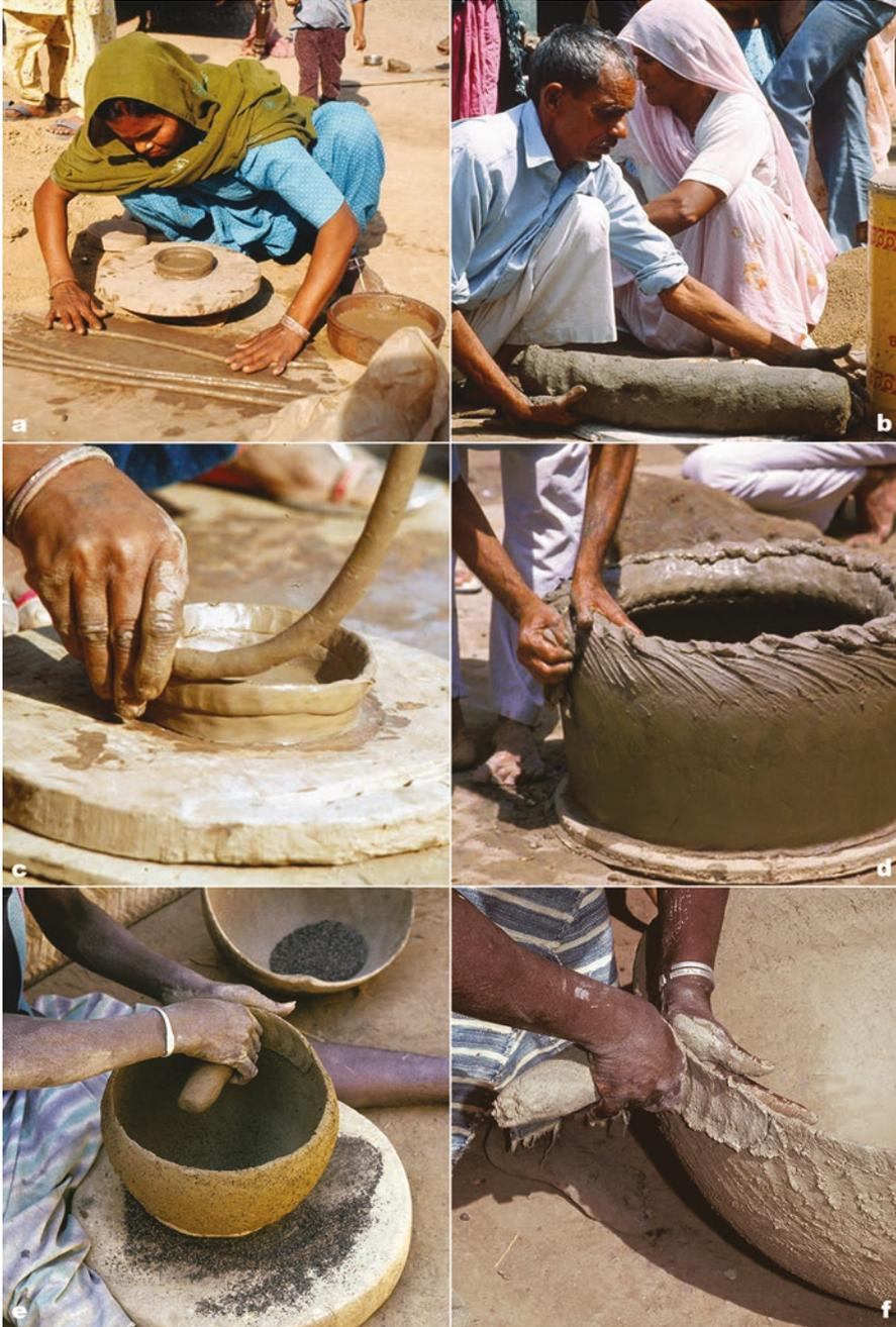
**Fig. 2.16** Coiling techniques: (a) and (b) forming coils by rolling an elementary volume of paste on a flat surface (Uttam Nagar, northern India); (c) coiling by pinching (Uttam Nagar, northern India); (d) coiling by drawing (Uttam Nagar, northern India); (e) and (f) coiling by spreading (Mali, ©A. Gallay)
