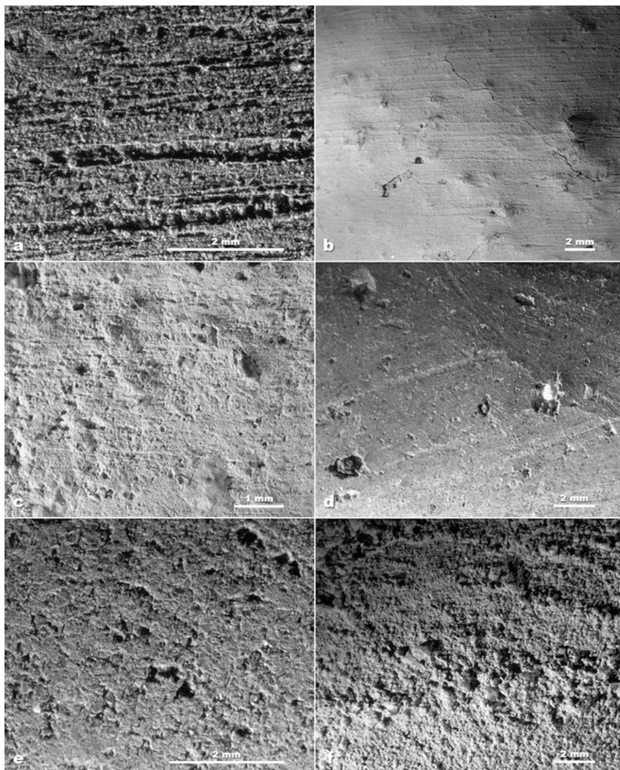
**Fig. 3.15** Granularity: (a) protruding grains; (b) totally covered grains; (c) partially covered grains; (d) floating grains; (e) inserted grains; (f) micro-pull-outs
