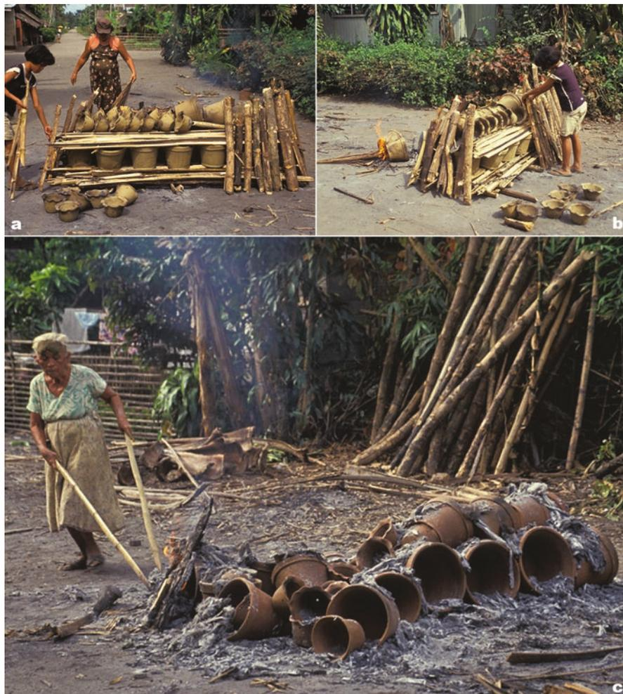
**Fig. 2.53** Firing on bamboo wattle (Leyte island, Philippines). After their pre-firing (b), the potteries are laid on racks made of bamboo poles against which bamboo poles are placed vertically (a). The firing lasts less than 20 min. The potteries are removed from ashes with long bamboo poles (c)
