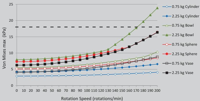
**Fig. 2.33** The Von Mises maximum values for the eight reproductions depending on the rotation speed ranging from 0 to 200 rotations/min. The threshold of collapse ( $18 \pm 2.7$  kPa) is showed by a dotted line
