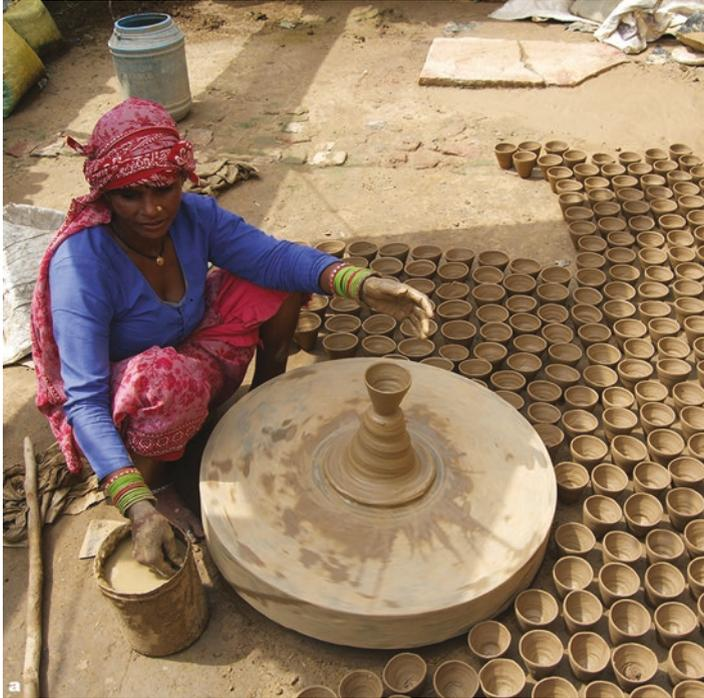
**Fig. 2.30** Wheel throwing off the hump (fly wheel, Uttar Pradesh, India)
