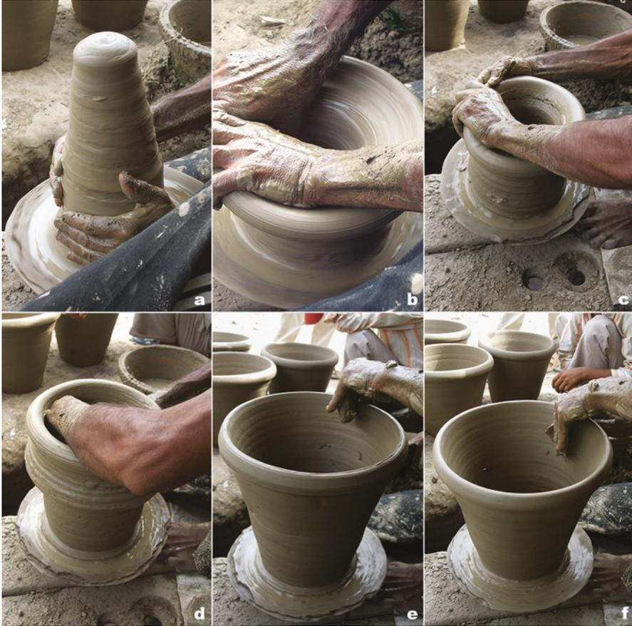
**Fig. 2.29** The different stages of wheel throwing: (a) centering; (b) hollowing; (c) and (d) thinning; (e) and (f) shaping (foot wheel, Uttar Pradesh, India)
