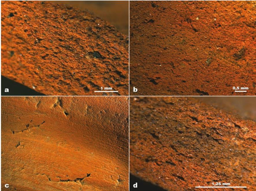
**Fig. 3.43** Diagnostic meso-structures of wheel throwing: (a, b) dense homogeneous meso-structure, random orientation and distribution of the coarse fraction; (c, d) tears due to a too fast rising of the interdigital pressures and abundance of the elongated vesicles parallel to the walls
