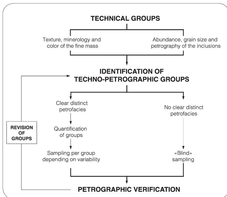
**Fig. 4.4** Techno-petrographic classification of ceramic assemblages
