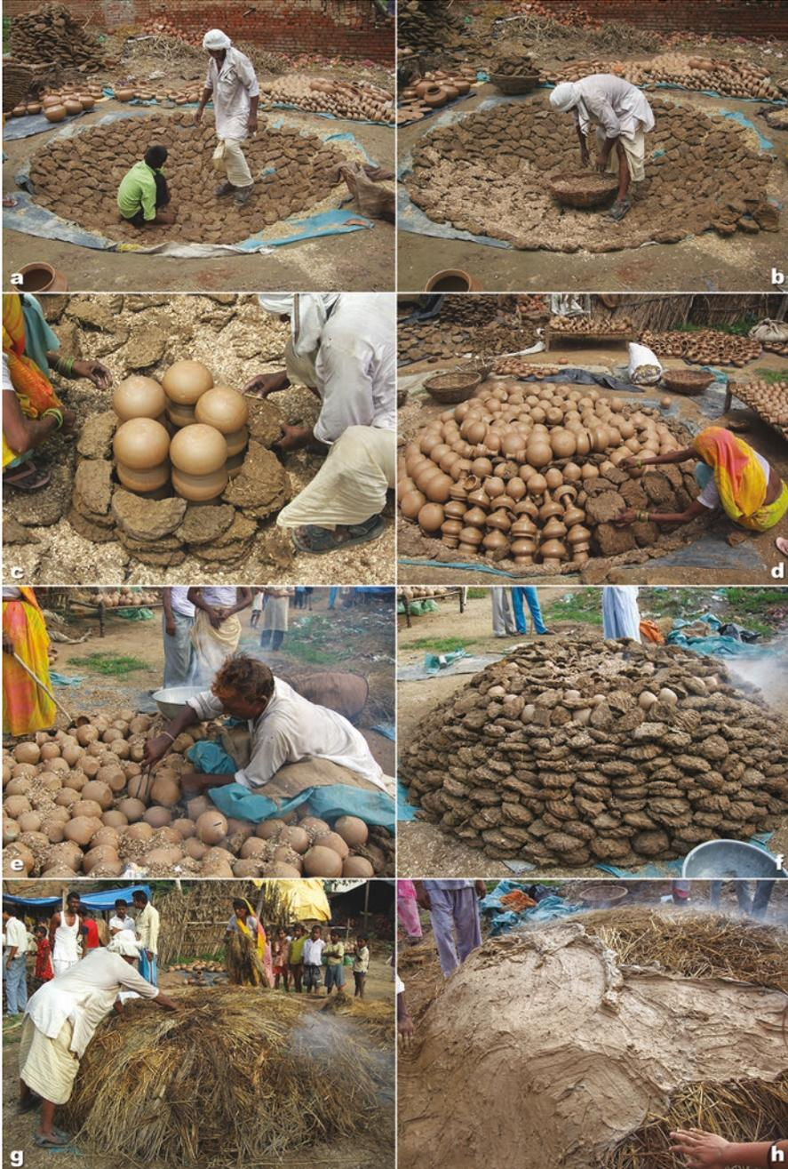
**Fig. 2.52** Open firing in depression: (a) and (b) dung patties and wooden dust are laid down in a depression covered by a plastic sheet; (c) recipients are piled to form a chimney; (d) the recipients are covered with cow dung patties; (e) the fuel placed at the bottom of the chimney is lighted; (f–h) the open firing is covered successively with dung patties, straw, and wet clay (Dibai, Uttar Pradesh, India)
