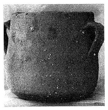
Fig. 93. Lime spalling on an unglazed vessel. Pieces of fabric are being dislodged by the white grains; others have already been removed (bottom center).
