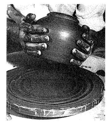
Fig. 60. Removing a vessel from a potter's wheel. Note the positions where marks may be left on the surface by the hands.
