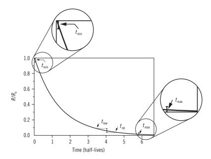
Figure 5.2 The limits of radiometric techniques for age estimation, displayed as a radiometric decay curve. The radioactive isotope ratio  $R/R_0$  decreases through time. Precision is shown by the vertical bar and the  $t_{\rm low}$ and t<sub>un</sub> age estimates. The maximum and minimum ranges are indicated when the error bars strike the 0 and 1.0 values on the y-axis, respectively (modified from Blackwell and Schwarcz 1993).
