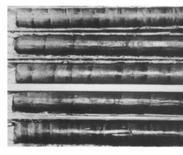
4.11 These cores bored from sedimentary lake deposits in Sweden show distinctive varves; each band of light to dark silt marks a single year's deposition of water-borne sediment. Varves vary in thickness from a few millimetres to several metres; these average approx. 2.5 cm. *Prof. D Tarling, University of Plymouth*
