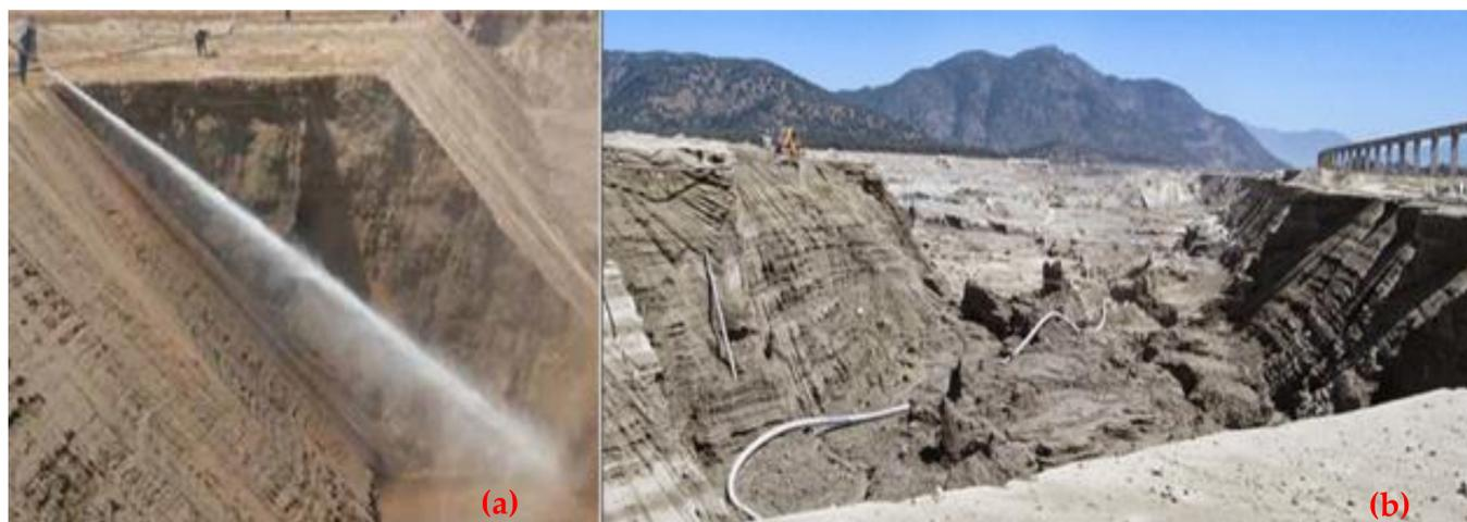
**Figure 26.** Tailings reprocessing by high-pressure water jets—Los Colihues TSF, El Teniente Mine. (a) High-pressure water jets operation. (b) Colihues TSF's reprocessing [43].
