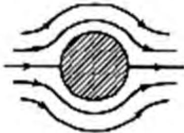
$$\bar{F}_{\text{arrastre}} = 6\pi\eta R v_0$$
