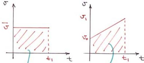
$$\bar{v} t_1 = v_0 t_1 + \frac{1}{2} (v_1 - v_0) t_1$$
