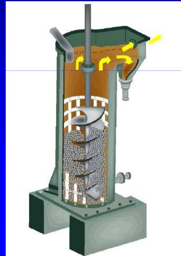
Figure 1. Schematic of Tower and Verti mill
