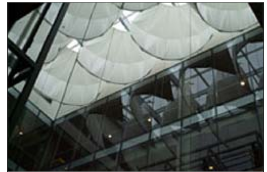
Interior office corridor overlooking atrium; Atrium sails control daylighting, solar gain, and glare
