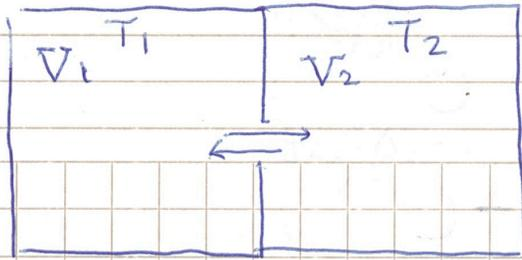
$$\frac{dN_1}{dt} = -A_1 \left( \frac{N_1}{V_1} \right) \frac{\langle v \rangle_1}{4} + A_2 \left( \frac{N_2}{V_2} \right) \frac{\langle v \rangle_2}{4}$$
