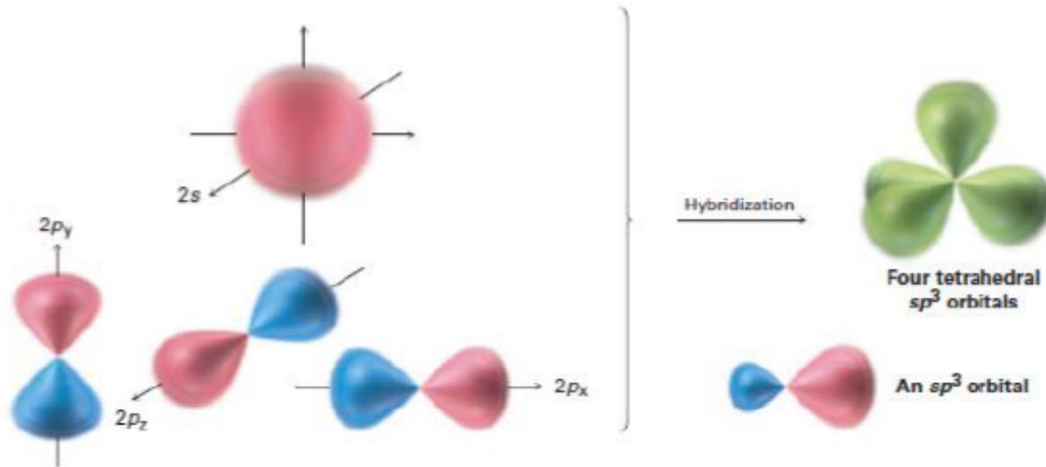
**Figure 1.10** Four  $sp^3$  hybrid orbitals, oriented to the corners of a regular tetrahedron, are formed by combination of an  $s$  orbital and three  $p$  orbitals (red/blue). The  $sp^3$  hybrids have two lobes and are unsymmetrical about the nucleus, giving them a directionality and allowing them to form strong bonds when they overlap an orbital from another atom.
