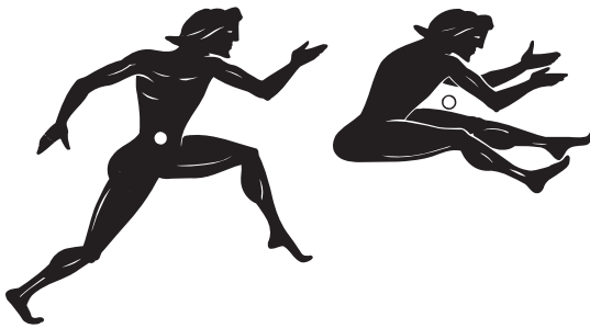
FIGURE 4.20 Center of mass. The single point at which the mass of a body can be thought to be concentrated is the center of mass. As the configuration of this jumper's body parts changes from takeoff (left) to midair (right), the instantaneous location of the center of mass (white dot) changes as well. In fact, note that the center of mass lies momentarily outside the body. A high-jumper or pole-vaulter can pass over the bar even though his or her center of gravity moves under the bar.
