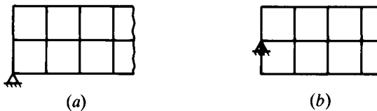
Figure 11.24 Modelling of a simple support.
