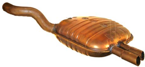
Fig. 19.6 Production series main muffler. The inner structural parts of the main muffler are removed
