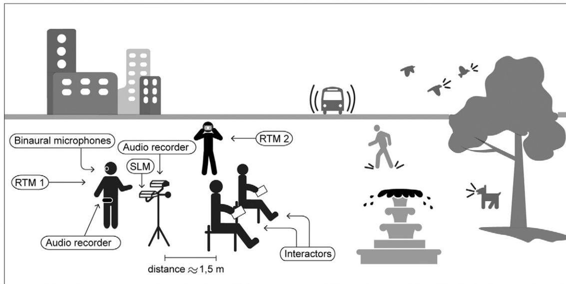
Fig. 3. Layout of the data collection scene in the environment, including the suggested position and orientation of the research team members (RTMs) and the instruments.
