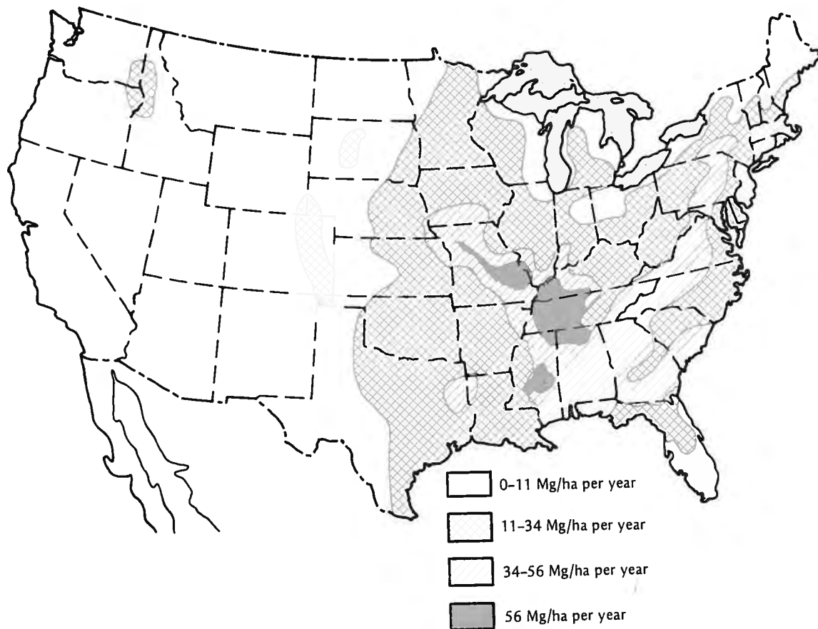
FIGURE 16.1 Extent of water erosion (sheet and rill) in continental United States in 1977. Gully erosion is not included. For the average soil, erosion rates greater than 11 Mg/ha per year will result in soil productivity decline. [From USDA (1975).]
