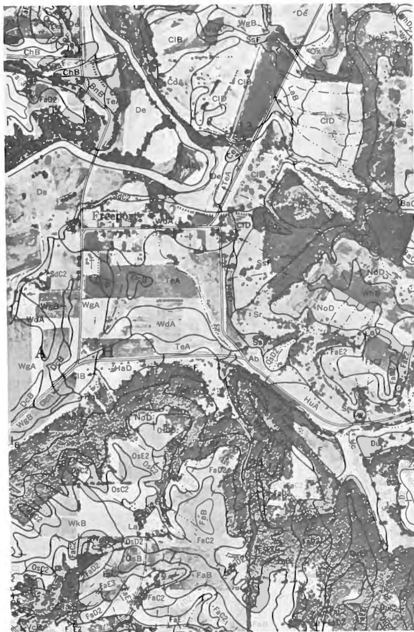
FIGURE 13.20 Field examination makes possible the delineating of soil boundaries, which are then indicated on the aerial photo (Figure 13.18). The soil legend identifies the soil name (first two letters), the slope (second capital letter), and the degree of erosion (the number). Thus, OsC2 is an Orwood silt loam (Os) that has a 5-9% slope (C) and is moderately eroded (2). [Courtesy USDA Soil Conservation Service, Soil Survey Staff.]
