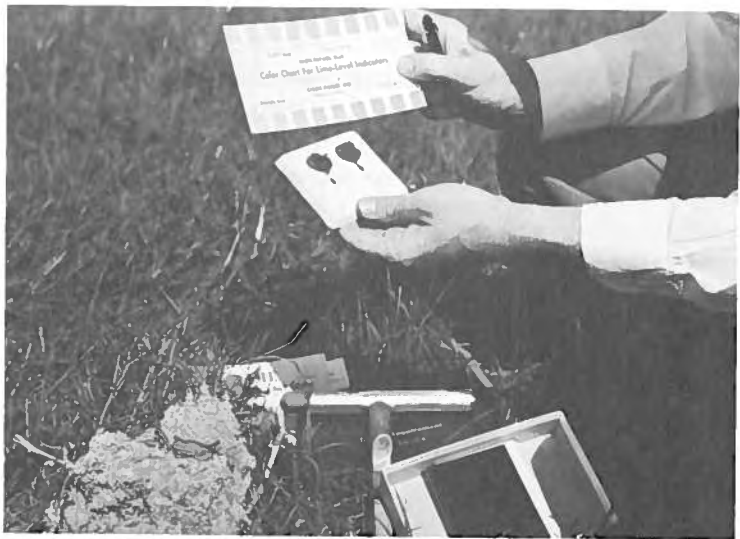
FIGURE 6.13 The indicator method for determining pH is widely used in the field. It is simple and is accurate enough for most purposes. [Courtesy New York State College of Agriculture and Life Sciences, Cornell University.]
