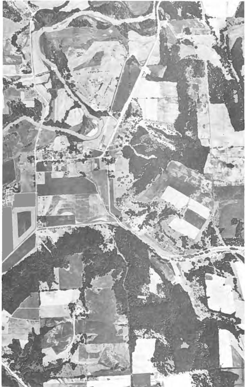
FIGURE 13.18 Soil survey maps are made using aerial photographs such as this one from Winneshiek County, Iowa. The field soil scientist is able to visualize quickly the topographic features of the section in which he is working. [ Courtesy USDA Soil Conservation Service, Soil Survey Staff. ]
