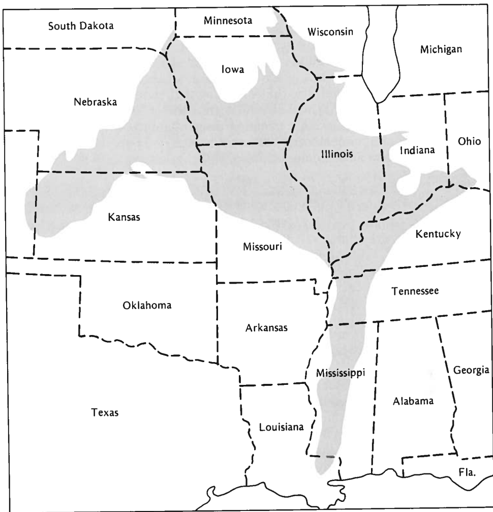
FIGURE 12.14 Approximate distribution of loess in central United States. The soil that has developed therefrom is generally a silt loam, often somewhat sandy. Note especially the extension down the eastern side of the Mississippi River and the irregularities of the northern extensions. Smaller areas of loess occur in Washington, Oregon, and Idaho (see Figure 12.11).
