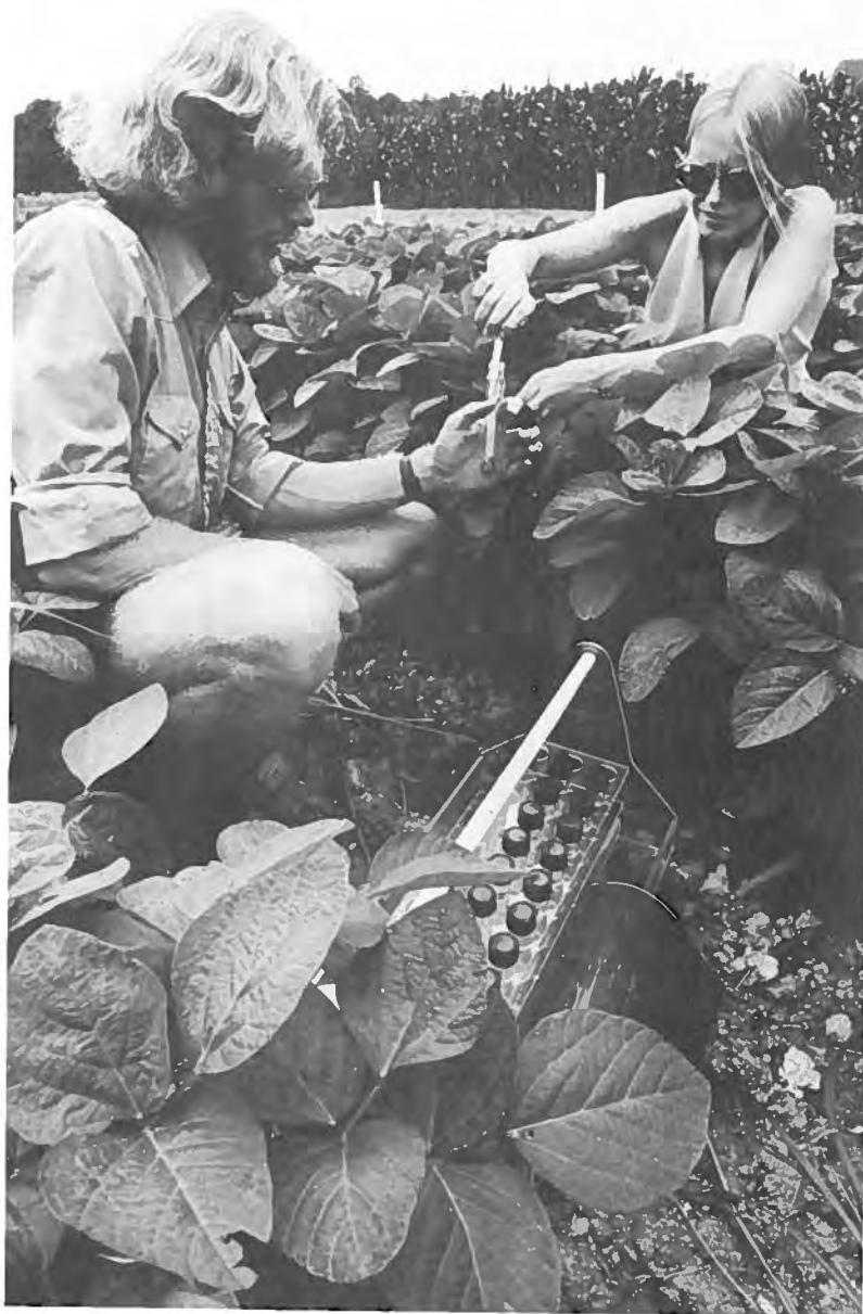
FIGURE 20.8 Collecting soybean leaf samples from a field fertilized with sewage sludge. The samples are to be analyzed for their heavy metal content, thereby helping to establish the levels of these metals in sludge that can be tolerated. [USDA photo by R. C. Bjork.]
