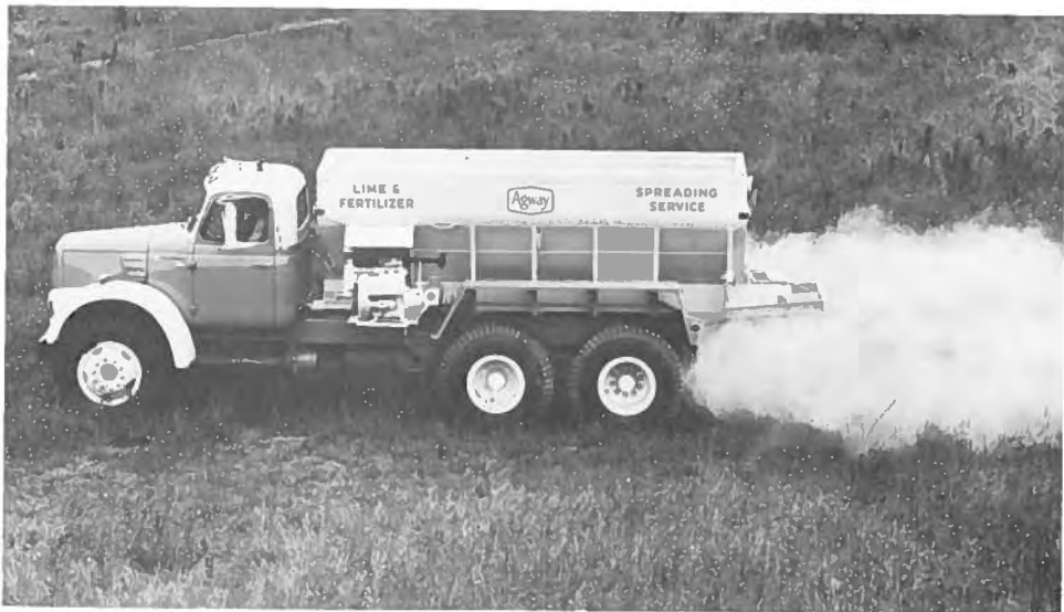
FIGURE 17.5 Bulk application of limestone by specially equipped trucks is becoming more and more common. Because of the weight of such machinery, much limestone is applied to sod land and plowed under. In many cases this same method is used to spread commercial fertilizers. [Courtesy Harold Sweet, Agway Inc., Syracuse, NY.]
