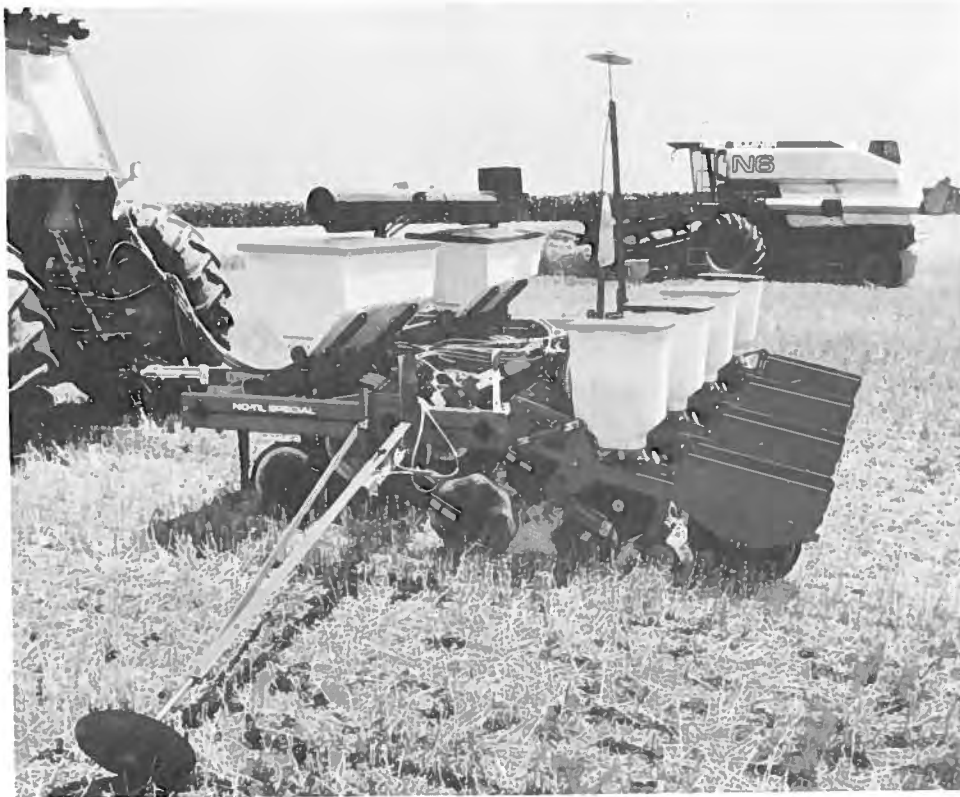
FIGURE 2.17 An illustration of one conservation tillage system. Wheat is being harvested and soybeans are planted with no intervening tillage operation. This no-tillage system permits double cropping, saves fuel costs and time, and helps conserve the soil. [Courtesy Allis-Chalmers Corporation.]
