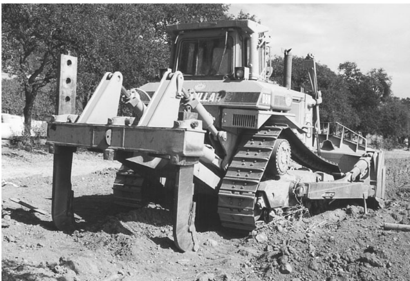
Figure B8.4.1 D8 “Caterpillar” with deep ripping shanks. Photograph by the author.
