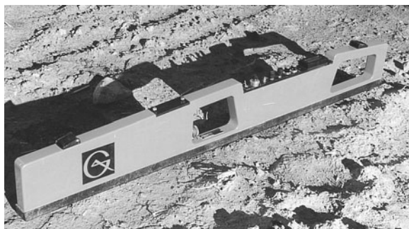
Figure B7.2.1 An EM38 salinity sensor. Photograph by the author.
