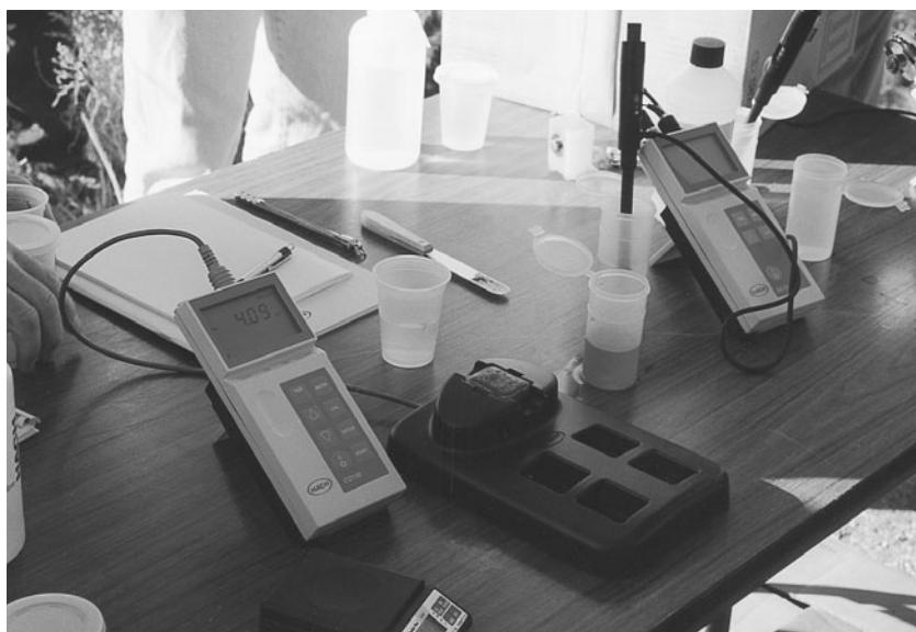
Figure B4.6.1 A portable pH meter with electrodes in a soil suspension. Photograph by the author. See color insert.
