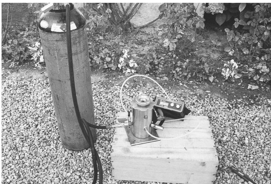
Figure 6.7 A pressure chamber for measuring leaf water potential. Photograph by the author.
