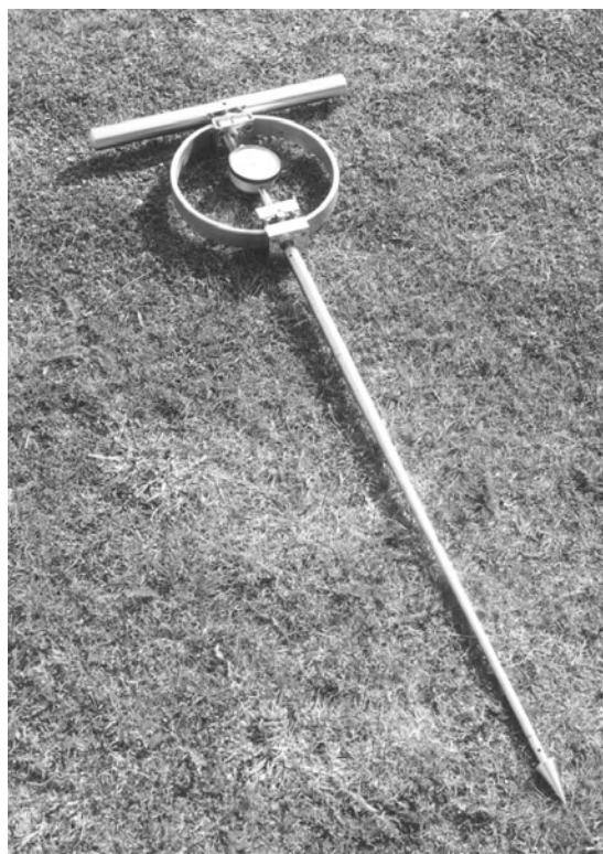
Figure B7.1.1 A cone penetrometer for measuring soil strength (White 1997, courtesy of D.B. Davies). Reproduced with permission of Blackwell Science Ltd.
