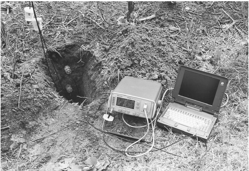
Figure B6.9.1 TDR probes, with Tektronix cable tester, installed in a vineyard soil. Photograph by the author.
