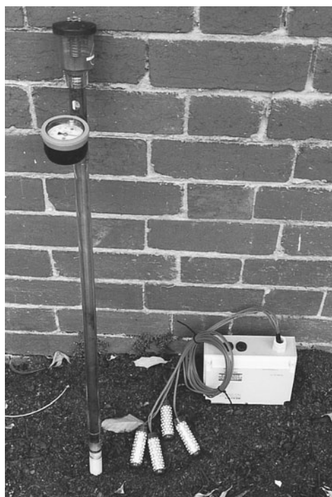
Figure B6.3.1 A tensiometer with vacuum gauge and a set of “Lite” gypsum blocks. Photograph by the author.
