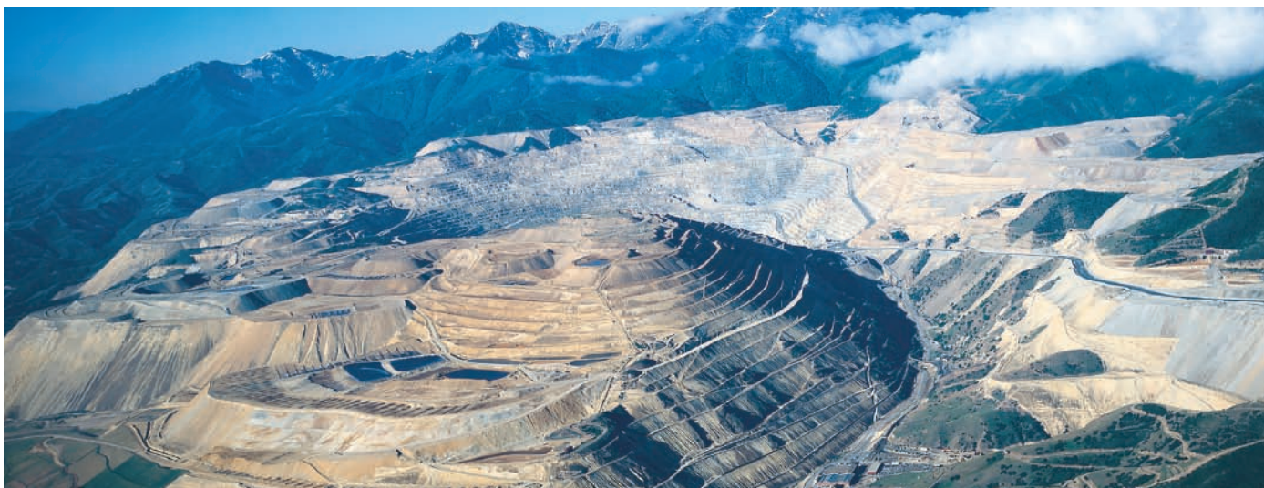
FIGURE 24.4 Porphyry copper deposits form around shallow igneous intrusions where hydrothermal fluids deposit copper and alter the surrounding rocks. Most are mined as large open pits with huge tailing (waste rock) piles like these near Bingham, Utah.
